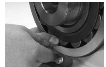
After mounting, the RIC should be checked at the unloaded roller.
